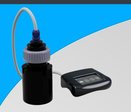
With the Photonic Measurements UV254 Dip Probe measure Natural Organic Materials (NOMs) at the remote locations and open water with a full colour portable IP65 display unit. The portable dip probe is submerge into water to perform surrogate measurements of TOC, BOD and COD without the need of expensive ragents. Measuring UVA, UVT and SUVA\* for responsive detection of aromatic organic material allows you to act on disinfection by-products such as Trihalomethanes (THM).
